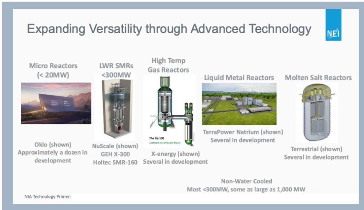
Figure 2. Types of Advanced Nuclear Reactors
